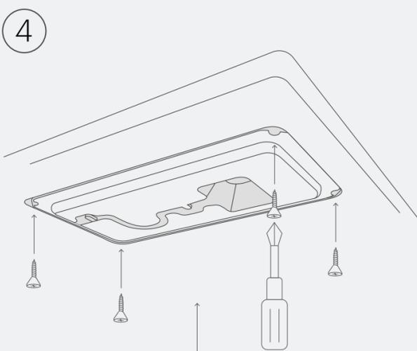
Use the four screws to fasten the Liberty built-in in the recess.
