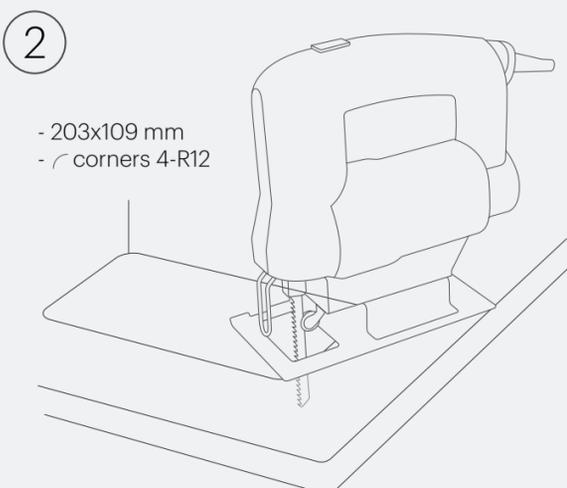
Use the jigsaw and follow the drawn lines to cut out the correct shape.
